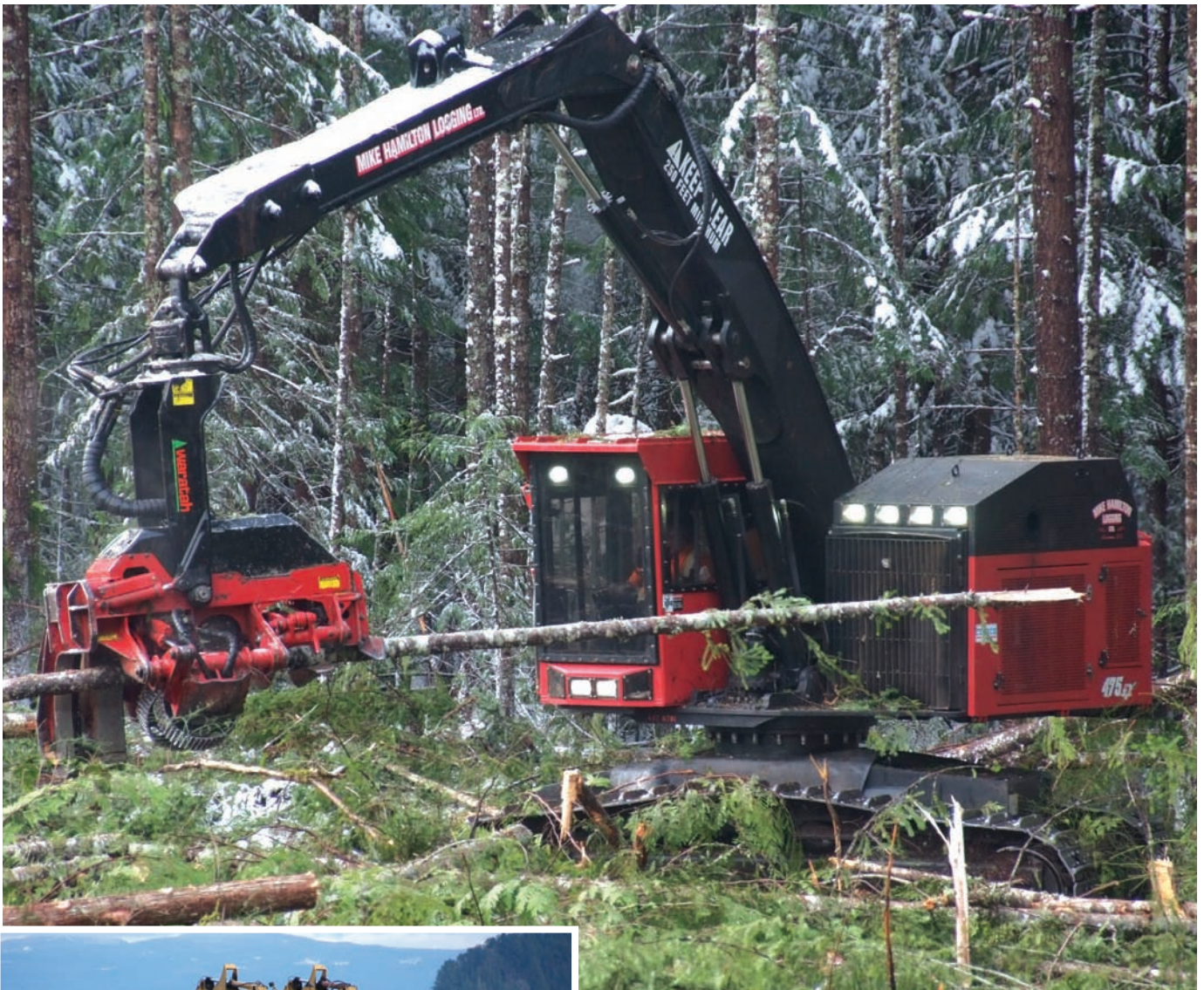
Above: A Valmet 475EX equipped with a versatile Waratah head processes small wood on a privately owned block just outside of Courtenay, BC on Vancouver Island. Left: A Wagner 120 stacker moves logs at the Union Bay Industries Dryland Sort, which is partially-owned by Mike Hamilton. The sort is located just a few Kilometres south of Courtenay on Vancouver Island.
